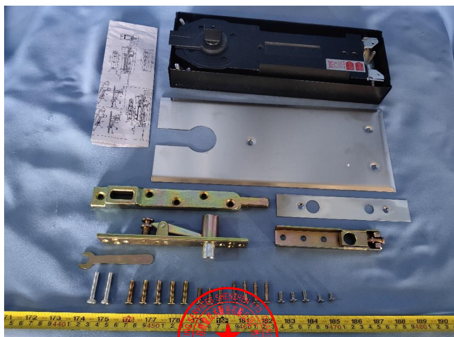
The cover plate after 24 hours of salt spray test
